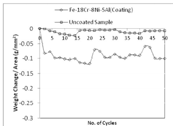
**Fig. 5.** Plot for weight change/area for uncoated and coated steel.
