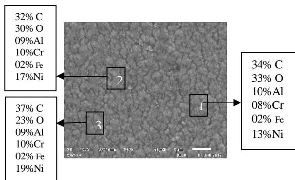
**Fig. 7.** SEM/EDAX analysis for oxidised Ni-Cr-5Al coating sprayed by PEMS technique on SS304L steel.
