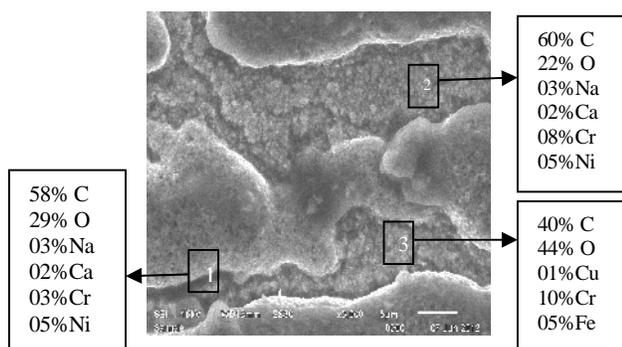
**Fig. 6.** SEM/EDAX analysis for oxidised uncoated SS304L steel.
