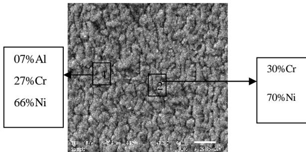
**Fig. 1.** SEM/EDAX analysis for Ni-Cr-5Al coating sprayed by PEMS technique on SS304L steel.
