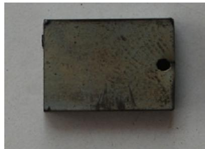
**Fig. 4.** Macrograph of Fe-18Cr-8Ni-5Al coated steel subjected to oxidation in air at 750°C.
