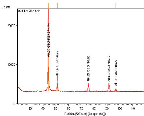
**Fig. 2.** XRD pattern for as-sprayed Ni-Cr-5Al coating.
